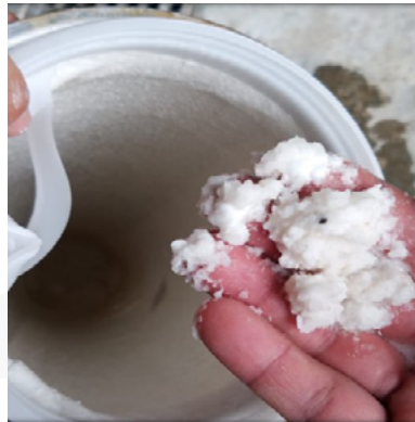
Disintegrated gypsum scale collected in the bag filters.
