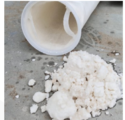
Disintegrated gypsum scale collected in the bag filters.
