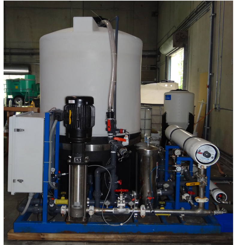
Membrane performance is evaluated using a single-element test skid at each stage of the cleaning study
